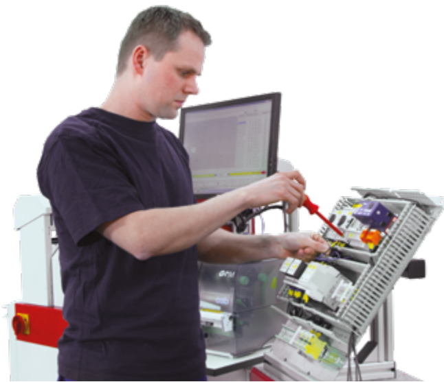
PWA 5000 can be used real-time during panel wiring. While the operator makes terminations, PWA is making the next wire to be installed.
