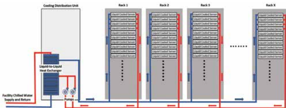
Integrated Rack Cooling Distribution Units (CDUs)
