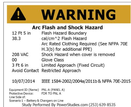
Figure 1. Example of Arc Flash Warning Label
