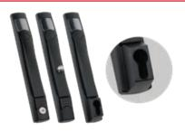
Flush Handles are optional for any solid, window or disconnect door that includes 3-point latching. They are ergonomically designed to provide style and function in a low profile. The handle is die-cast zinc finished with RAL 9005 textured black polyester powder paint. Provision to add your logo is included. Handle can be installed to rotate either clockwise or counterclockwise.
