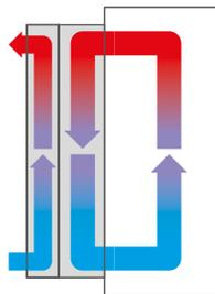
In closed loop cooling, the sealed integrity of the cabinet will be maintained with either an air conditioner or heat exchanger, protecting the equipment from dirt, dust, corrosive air and wind-driven rain. Any holes or cutouts in an enclosure must be filled with a device that has the same (or better) Type rating. The enclosure takes the rating of the lowest rated component
