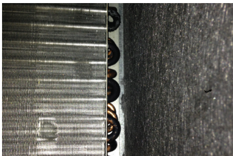
Figure 2. Coil failure inside of an enclosure through the effects of moisture and corrosion.
