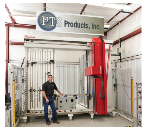
Paul Soberg, founder of Minnesota-based panel shop PTS Products, achieved higher quality and faster turnaround times by automating custom cutouts on its enclosures and back panels using the Steinhauser ModCenter.
