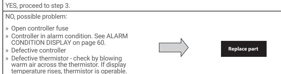
3. The cooling status indication (symbol G) should be on. Is the symbol on? If not, press and hold the lower right "snowflake" button for greater than five seconds. Is the cooling mode symbol now on?
