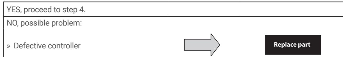
4. The evaporator (Enclosure or "COLD" air) fan/impeller should turn on. Is there airflow?
