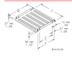
Fixed Shelves mount to the front and back 19-in. rack angles. The shelf is 2,0 mm steel with adjustable 2,5 mm steel supports. Adjustable to fit multiple-depth enclosures or rack angle placements. Entire assembly is finished with RAL 7035 textured, light-gray polyester powder paint. Load rating is 68 kg.
