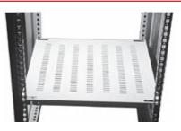
Vented Frame Shelf mounts to the vertical hole pattern on a frame and provides a stationary surface for equipment. The shelf is 1,5 mm steel finished with RAL 7035 textured, gray polyester powder paint.
