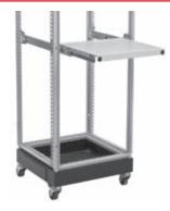
Frame Pull-Out Shelf allows easy access to shelf-mounted devices. The shelf is 1,5 mm steel with 2,0 mm steel supports. The entire assembly is finished with RAL 7035 textured, gray polyester powder paint. The shelf mounts to the front and rear frame uprights. Mounting hardware included. Load rating is 50 kg.
