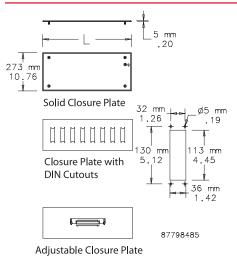
Closure Plates seal the ends of the cable entry cabinet. Made from 2,0 mm steel and finished with RAL 7035 textured gray polyester powder paint.
