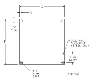
One-piece mounting foot kit consists of the necessary hardware to attach two fiberglass feet, molded from the same material as our A48 enclosure. This compression-molded fiberglass material has excellent chemical and temperature resistance and provides outstanding performance and durability in harsh environments. The mounting feet can be field installed on either the 18x16 or the 20x16 enclosure.
